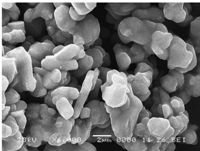
Fig. 2. A typical SEM image of \text{LiM}_{0.02}\text{Co}_{0.98}\text{O}_2 powders.
